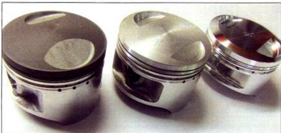
Don't new pistons look nice - these ones represent sizes for 510cc, 553cc and 587cc and there's even more!
