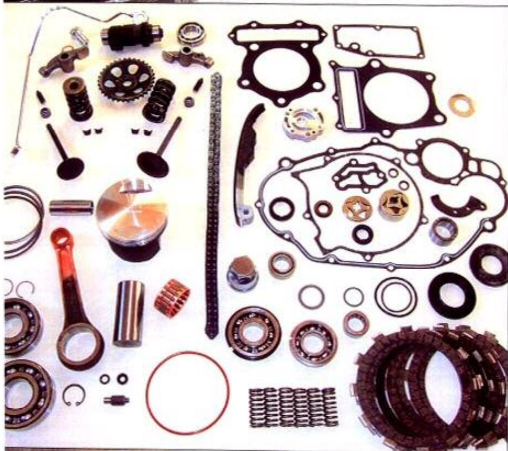
This is our minimum layout of parts that are required for Stage 1 rebuilds and it should be your minimum too.
